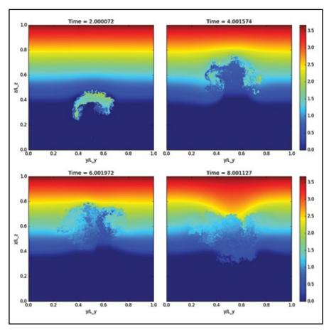
Example evolution of the buoyancy in a simulation with 864<sup>3</sup> grid cells
