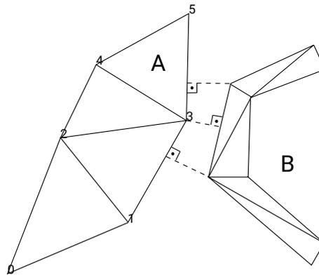
Figure 1: Two meshes  $A$  and  $B$  are checked against each other. An enumeration for the vertices of  $A$  is given. We denote the three shortest distances.
