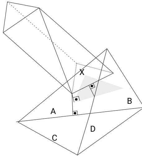
Figure 2: Geometric checks for a triangulated volume approaching a plane (at the bottom) spanned by four triangles A,B,C,D. The comparison of triangle X to A finds the contact point (shortest line) through a projection of a vertex of X onto A. Comparing X to C first obtains the same point projecting the vertex onto the plane spanned by C, but then it has to move the anchor point on the plane into C. When we compare X to B, the closest line is found between two edges.
