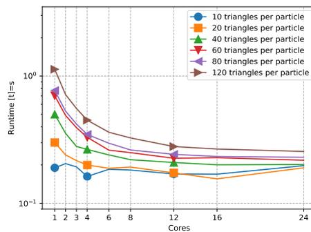
Figure 3: Scalability of the triangle-to-triangle comparisons in a DEM context where two particles collide. From [2].
