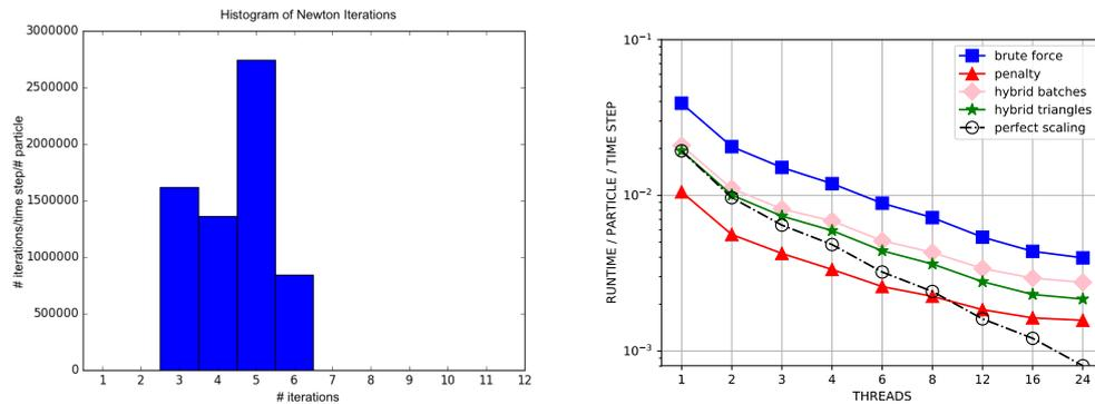
Figure 4: Left: Typical number of required Newton iterations if we equip the iterative scheme with a dynamic termination criterion. Right: Scalability of three core comparison approaches. From [4] and [2].
