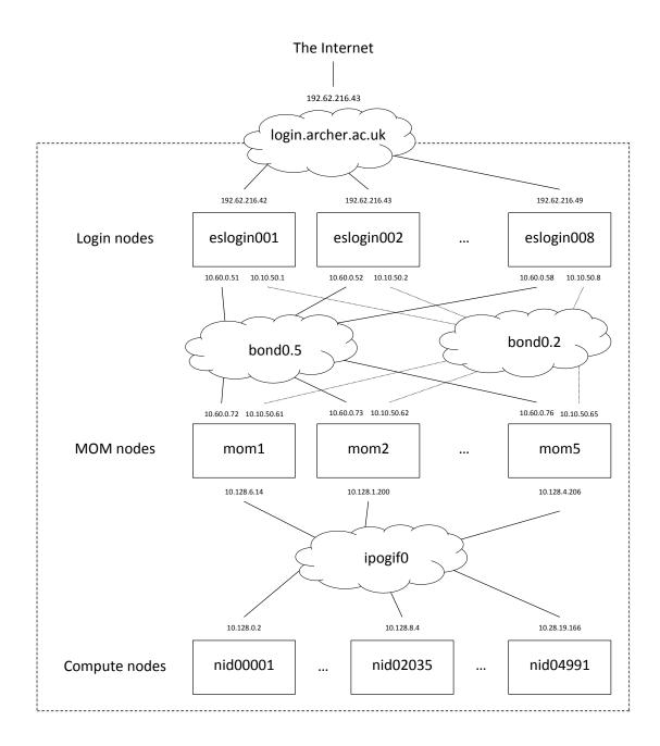
Figure 1: Schematic of ARCHER network connectivity
