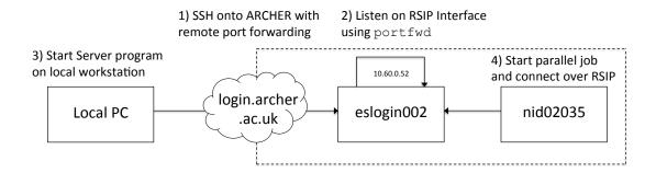
Figure 3: SSH tunnelling in combination with RSIP on ARCHER
