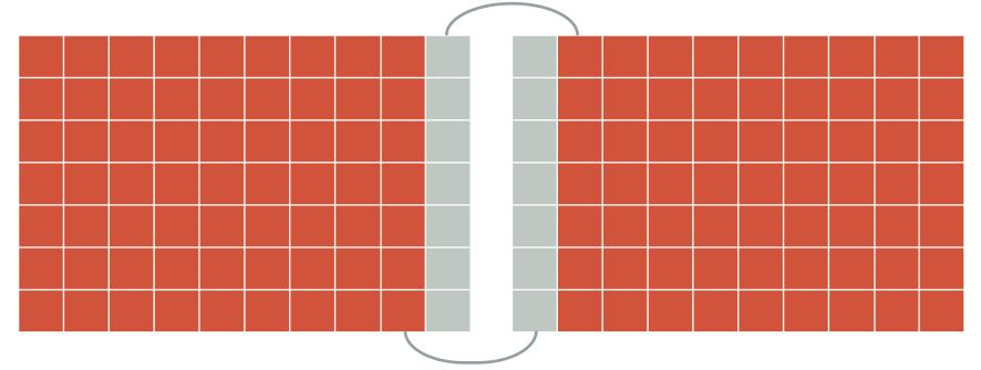
Halos transferred via MPI\_Sendrecv
